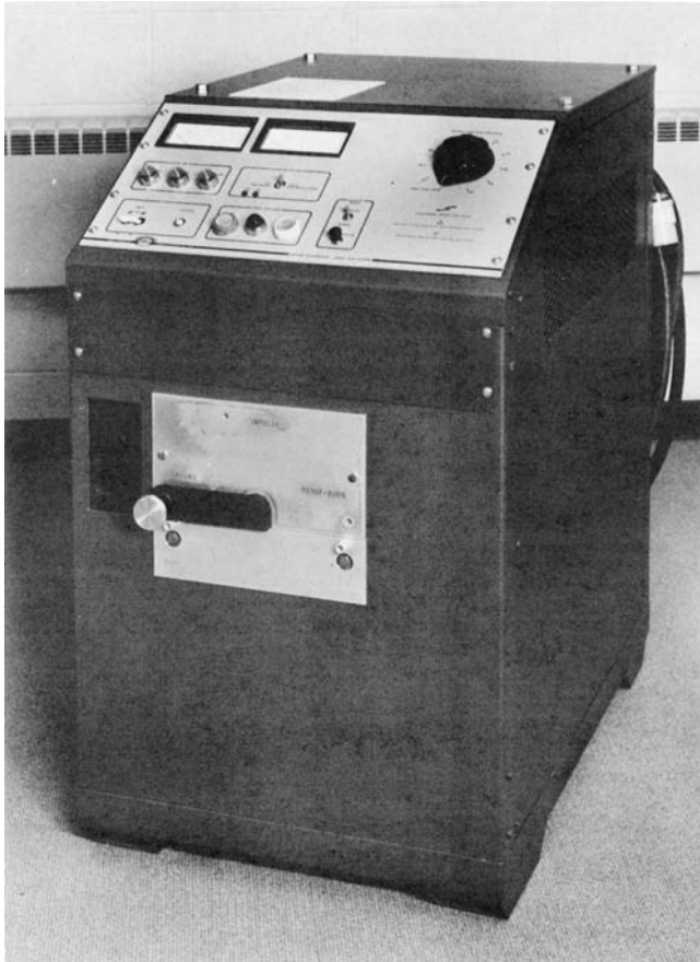
FIGURE 5.43 Heavy-duty cable test and fault-locating system. (Courtesy of James G. Biddle Company.)
